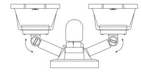
Both lamp heads can be rotated 180º left and right. Adjust these parts and joints to reach optimum angle and range of illumination.
